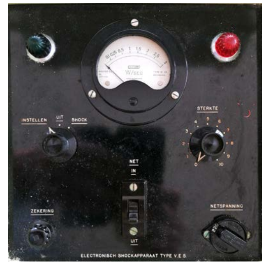
Electric shock apparatus with control panel, built in the Netherlands, probably in the 1950s (9 kg, dimensions 21x23x36 cm).
