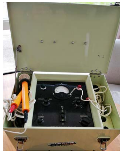
Electric shock apparatus with control panel, built in the Netherlands, probably in the 1950s (9 kg, dimensions 21x23x36 cm).
